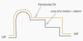
Two CTs measure the load differential between two groups of motors loads; when a motor is lost, the differential increases and the sensor alarms.
